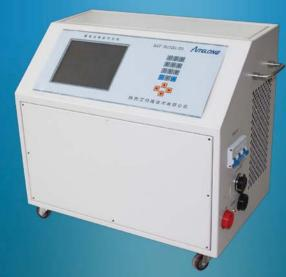
SAT-DC200 series Full-automatic battery charger has an intelligent three-step charging mode, which realizes the switch between equalized charging and floating charging, and that between constant current and constant voltage automatically as well as sets and controls the parameters such as voltage, current. It has a LCD screen and all-English menu, making the operation easy and the intellectualization excellent.
